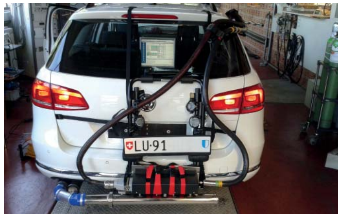
PEMS: portable emissions measurement system
