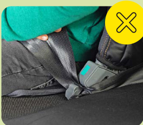
Incorrect belt routing – the child is not optimally protected.
